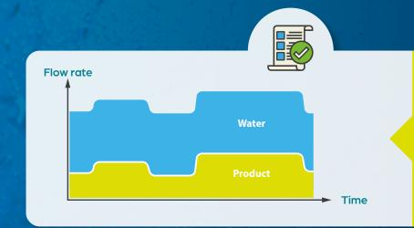
In contrast to other medication methods, the new **MD Advanced** ensures consistent **linear dosing** at all times, as shown in the image.
